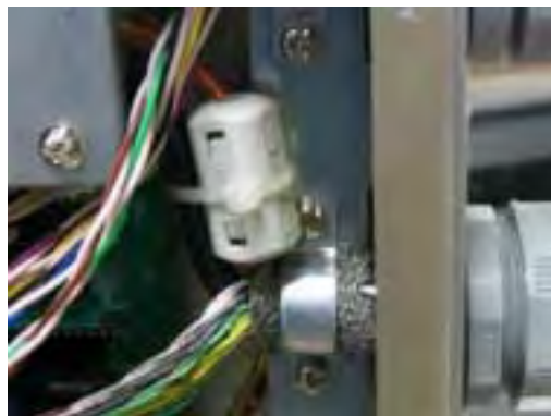
Attaching EMI core RFC-4
